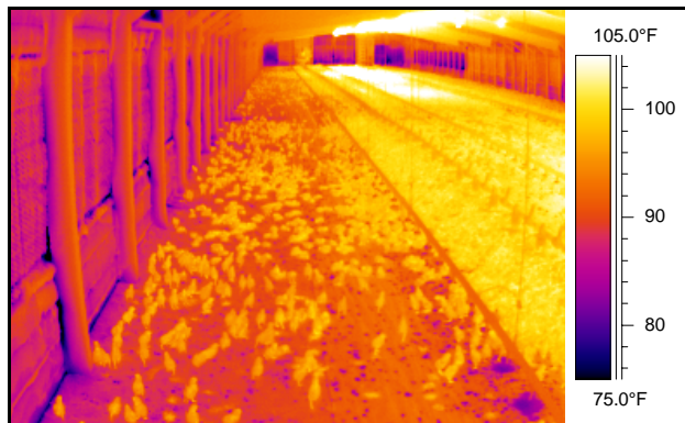
Figure 6. Thermal image of two-day-old chicks in spray foamed house with radiant tube heaters.
